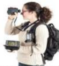
Example of modern equipment for surveying (Field-Map technology): GPS, laser range finder, and field computer allows surveying as well as cartography (Creation of map in real-time) and field data collection.
