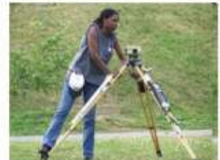
Center for Operational Oceanographic Products and Services staff member conducts tide station leveling in support of the US Army Corp of Engineers in Richmond, Maine
