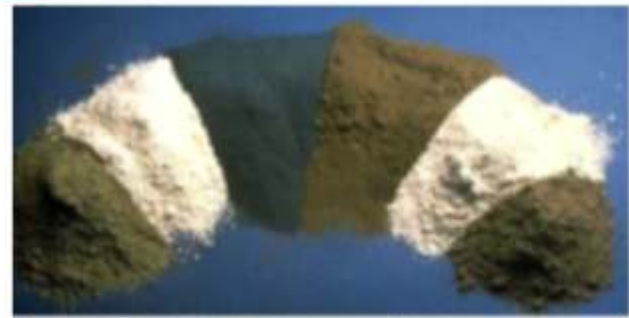
Figure 13: Green Substitutes to Cement known as supplementary cementitious materials (From the left to the right, class C fly ash, metakaolin (coloured clay), silica fume, class F fly ash, ground granulated blast furnace slag, and calcined shale)
